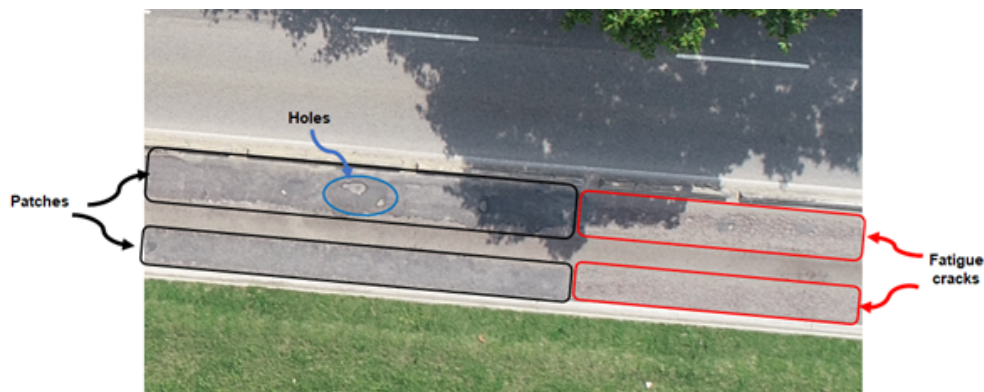
Figure 12 Presence of patches, potholes, and fatigue cracking in Section 01.
