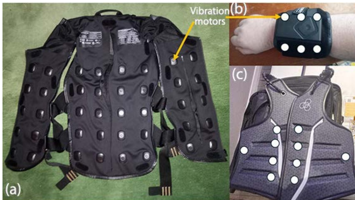
Figure 2: Example Haptic Devices: (a) bHaptics TactSuit x40 (features 4x5 grid of vibration motors on front and back); (b) bHaptics Tactosy for Arms (features 2 rows of 3 vibrations motors, shown by white dots) 1 abd (c) Actonika Skinetic (features 20 voice coil motors as shown by the white dots – the pattern is repeated on the back).
